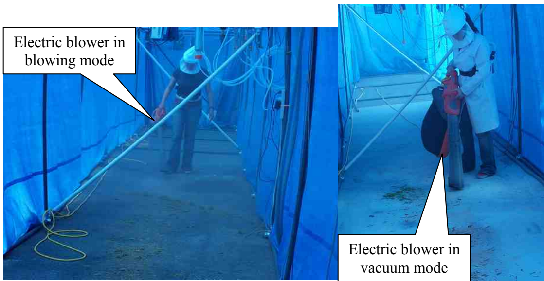
Figure 5. Electric powered hand held blower/vacuum.
