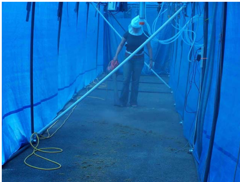
Figure 19. Blowing operation for horizontal gradient tests.
