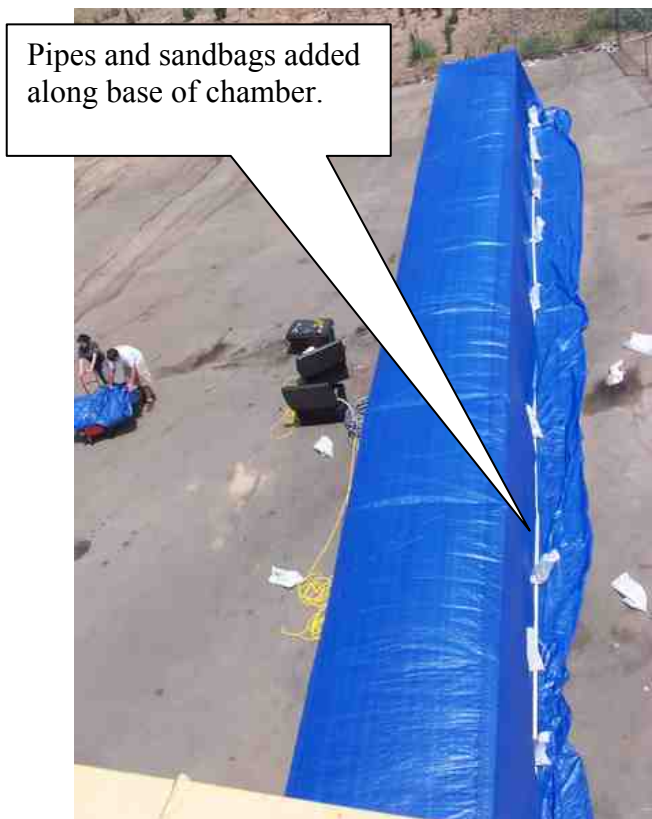
Figure 13. Addition of pipe and sandbags along base of chamber to eliminate leaks.
